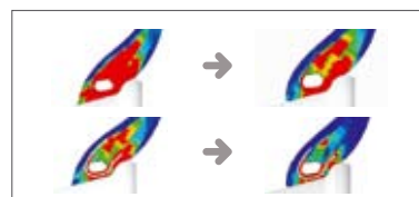
Improvement of Bead Durability Minimization of strain energy in bead portion
